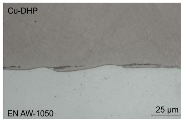
Figure 5 Cross section of a magnetic pulse welded joint
