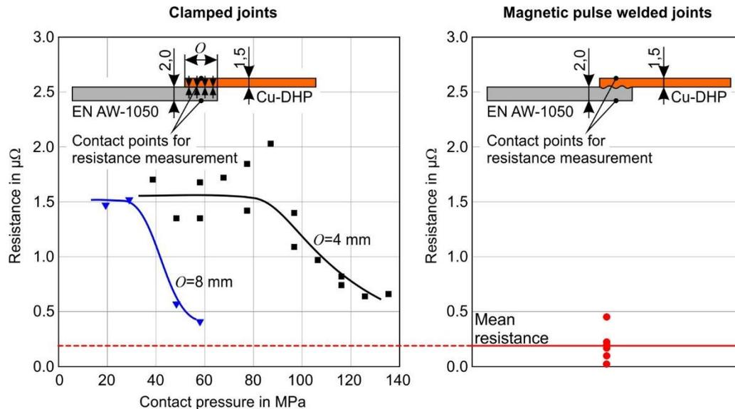
Figure 6 Electrical resistances of clamped (left) and magnetic pulse welded (right) aluminium copper joints
