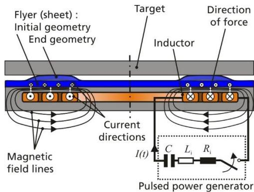
Figure 2 Process principle of magnetic pulse welding of tubes
