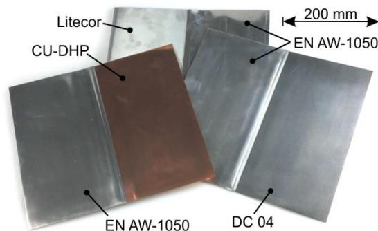
Figure 7 Magnetic pulse welded multi-material joints
