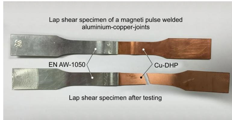
Figure 4 Lap shear test of magnetic pulse welded copper aluminium hybrid sheets
