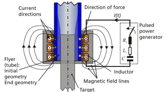
Figure 3 Process principle of magnetic pulse welding of sheet metal
