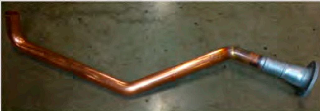
Cu-tube brazed onto a steel flange
