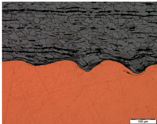
Figure 2. Wave formation in a copper-steel weld interface
