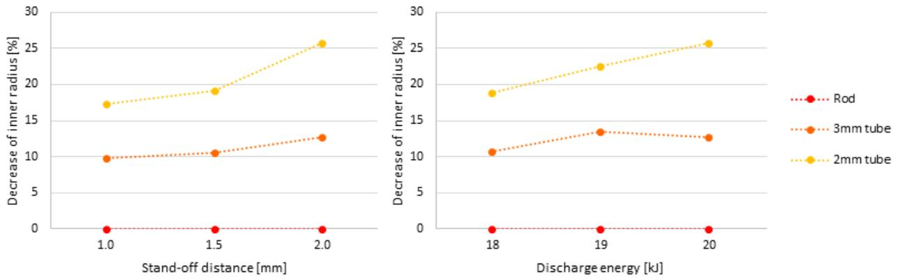
Figure 7. Decrease of inner radius of steel inner workpiece as a function of stand-off distance (left), discharge energy (right) and inner workpiece thickness
