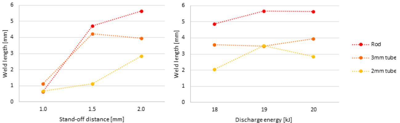
Figure 9. Weld length in function of stand-off distance (left), discharge energy (right) and inner workpiece thickness
