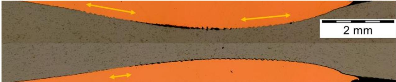
Figure 11. Top: Weld interface with 2 welded regions, opposite of the field shaper cut - Bottom: Weld interface with one welded region and a broken region at the field shaper cut
